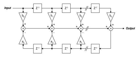
$Z^{-1}$  = Unit Time delay (sampling delay) a, b = simple gain blocks
